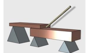
4. **Assembly.** The parts to be joined need to be placed together in such a manner that they are unlikely to move during brazing. Some angle iron can give a thin edge which will reduce heat being transferred to it. Bricks can raise the parts to allow the heat source to get underneath the are being brazed, as this will assist the capillary action of the molten filler rod. Rounded corners of the parts can also assist in the capillary action.
