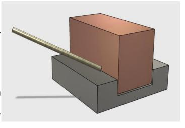
hotter area. The rule here is, the hotter the molten metal, the more fluid it is, so the more it flows into the joint. Imagine pouring water into a joint compared to honey. The water will run straight through, the honey won't.
