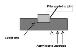
The brazing process functions by having the rod material become very fluid and flow into close fitting joints by capillary action. The parts being joined are heated, the filler rod is placed on the joint, and the heat from the parts melts the rod, sucking the liquid metal into the joint. If the rod is placed further away from the joint, there is a danger that the liquid material will just flow over the surface of the parts and not flow into the joint.
